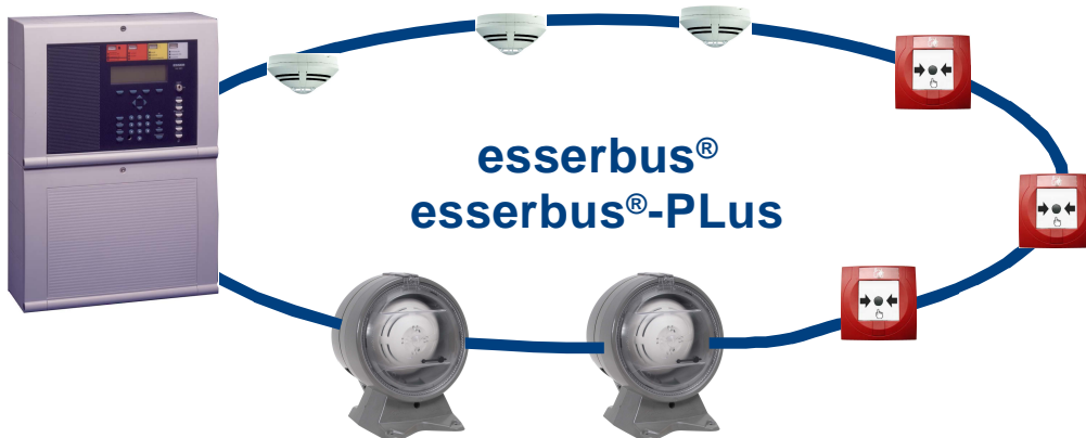
Fig. 52: Schematic circuit diagram of loop
