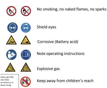
The hazard symbols on the left side correspond to ISO 7010. The hazard symbols on the right side correspond to the European industry standard EN 50342-1 for starter batteries. In dependence of the respective normative background the hazard symbols shown here are suitable to fulfill the safetyrelated requirements. A marking of batteries after GHS CLP-regulation is not required.
